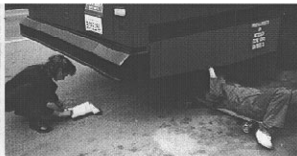
California Highway Patrol inspectors at the San Diego crossing conduct a level-1 inspection. The bus was placed on portable ramps to facilitate an undercarriage inspection.
