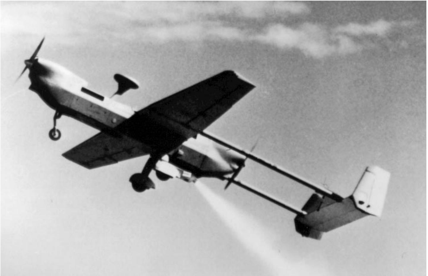
Each system includes eight UAVs with payloads, a launch and recovery station, ground stations for controlling flight and processing information from the UAVs, and other related equipment. (See fig. 2.) DOD plans to buy 24 systems for the Army, 18 for the Navy, 5 for the Marine Corps, and 3 for training, for a total of 50 systems.
