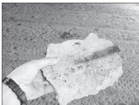
Source: GAO. Concrete that Fell from Flume
