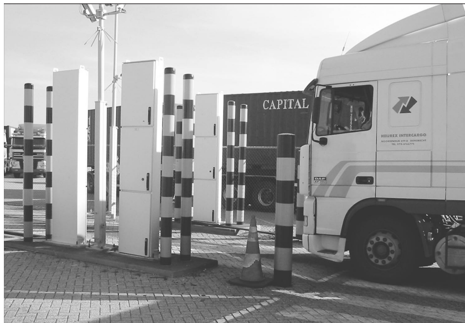
Figure 2: Truck Passing through a Radiation Portal Monitor in Rotterdam, the Netherlands
