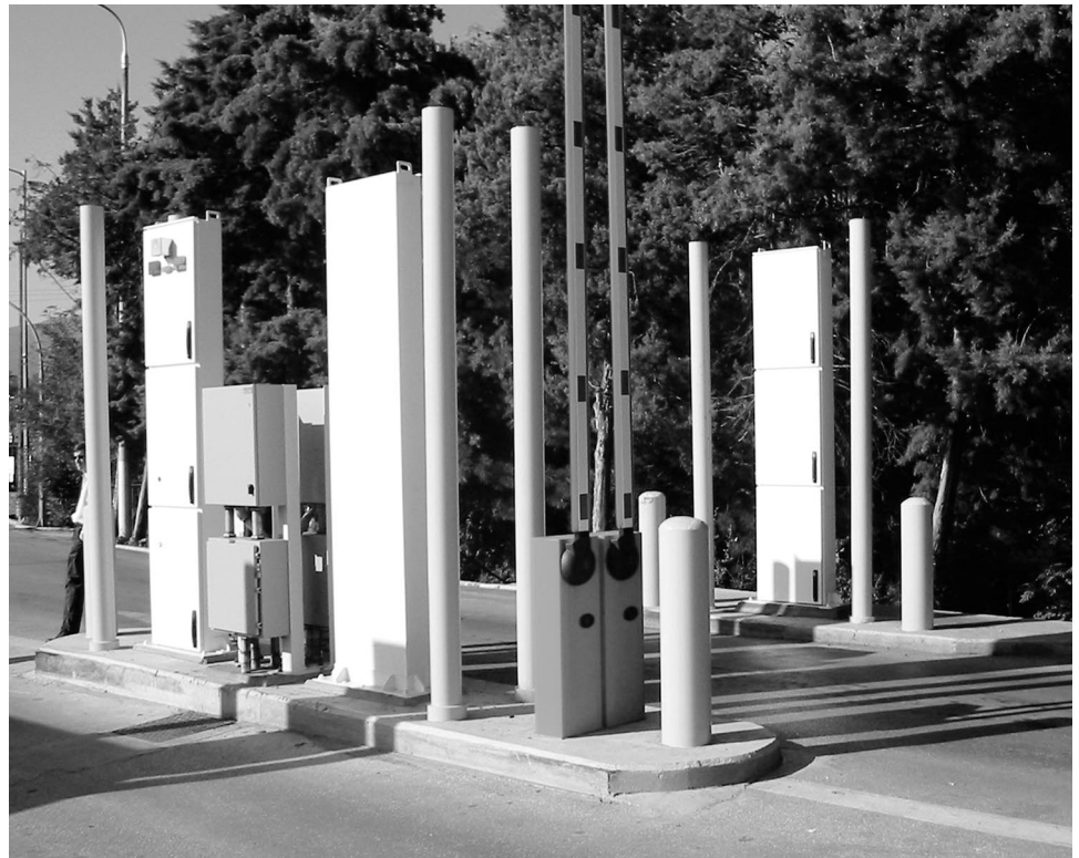
Figure 6: Radiation Portal Monitors at a Northern Greek Border Crossing
