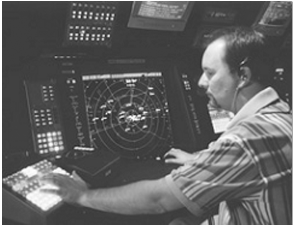
Figure 2: An Air Traffic Controller Uses a Digital Radar Display and Workstation Computers Interconnected through Telecommunications Systems for Air Traffic Management
