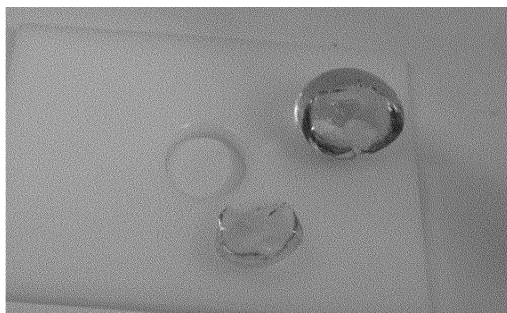
Figure 7: Expanded Water Bead After Being Fragmented by 10.0 mm Diameter Rod End.
