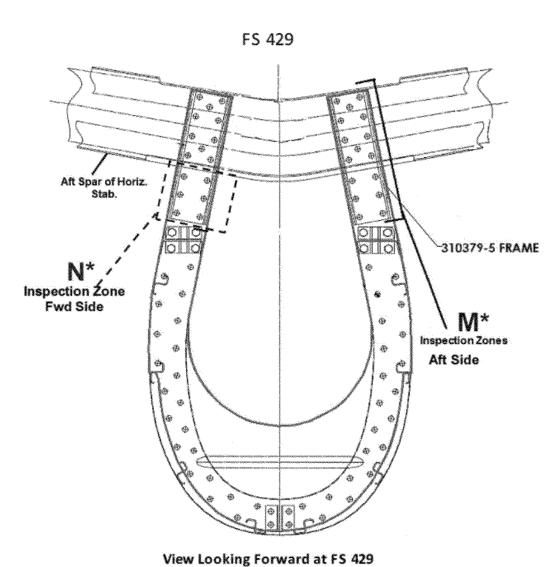
(M) FS 429: Aft Frame Channel and Web (\* inspection mirrored on opposite side)(N) FS 429: Forward Channel attached to Frame (\* inspection mirrored on opposite side)
