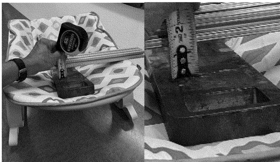
(xxii) 7.15.4 Using the equation shown in Figure 9 to this paragraph (b)(10)(xxii), calculate the concavity r by inputting the width L and depth D into the equation below. r values greater than 22 cm (8.66 in.) meet the concavity requirement.
