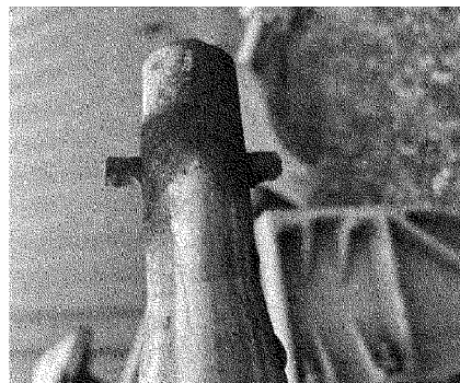
Figures 4,5,6-Heavily oxidized and worn king pin tabs
