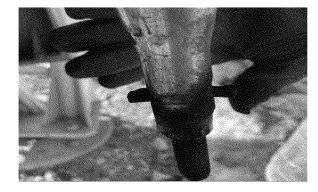
Figure 7-Roll pin crack on king pin
