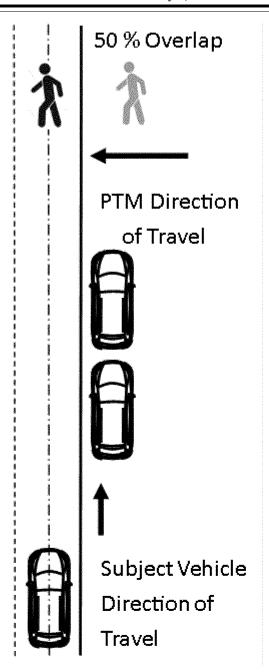
Figure 6 to § 571.127—Setup for Pedestrian Along-Path Stationary
