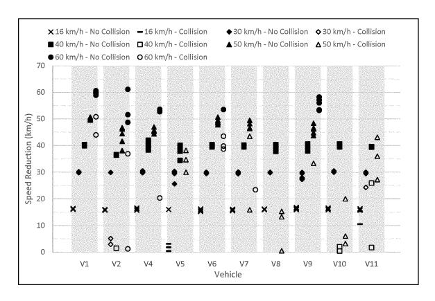
In the agency's crossing path from the right with 50 percent overlap during dark lighting condition using the vehicle's upper beam headlamps, one vehicle avoided collision in all but one test when tested at speeds up to 60 km/ h (37 mph), and another vehicle avoided collision on all tests at speeds above 20 km/h (12 mph) and on most tests at 16 km/h (10 mph). A total of four vehicles avoided collision either on all or some of the tests at 60 km/h (37 mph) and on
