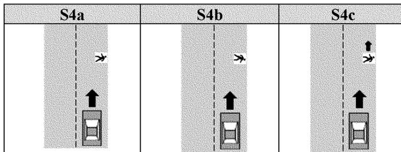
In the first scenario the stationary test mannequin is facing away from the vehicle (S4a) and in the second, it is facing toward the vehicle (S4b). In third scenario, a subject vehicle encounters an adult test mannequin walking in front of the vehicle on the nearside of the road away from the vehicle (S4c). In all three procedures, the stationary test mannequin is positioned with a 25 percent overlap from the passenger side of the vehicle.
