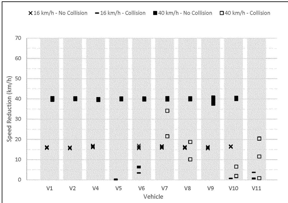
Even though testing was not performed at 60 km/h (37 mph) for the crossing path from the right and 25 percent overlap condition, based on the results observed at 40 km/h (25 mph) for the 25 percent overlap, NHTSA has tentatively concluded that the proposed performance testing requirements are practicable. The agency is currently performing testing at the proposed speed ranges, including the 60 km/h (37 mph) speed, to corroborate this conclusion. NHTSA is proposing a
