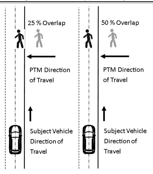
Figure 4 to § 571.127—Setup for Pedestrian, Crossing Path, Left
