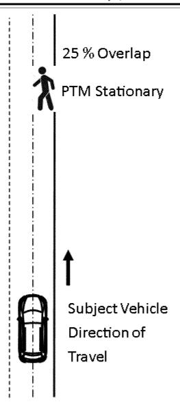
Figure 7 to § 571.127—Setup for Pedestrian Along-Path Moving
