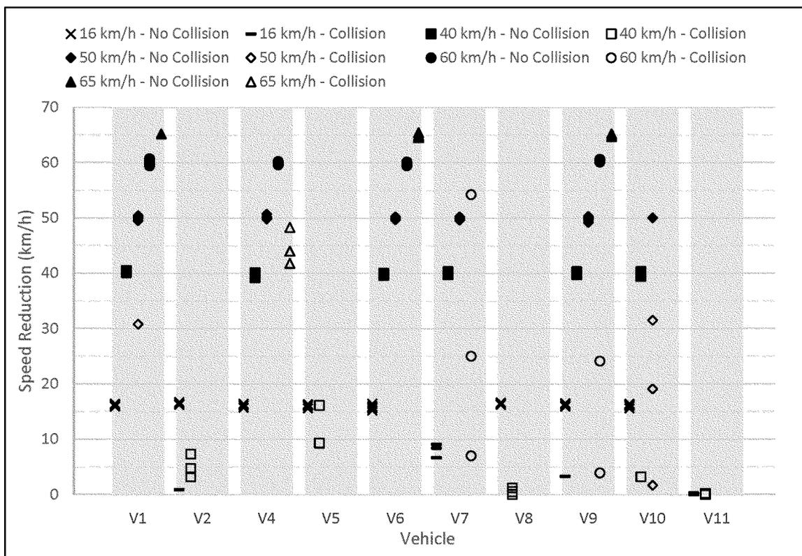
Testing for the dark upper beam along path pedestrian test mannequin moving scenario produced better performance than when testing for the dark upper beam stationary scenario. In the along path moving scenario, the test mannequin moves away from the subject vehicle at a constant speed and continues moving even as the subject vehicle decelerates during the AEB event. This has the potential to allow for
