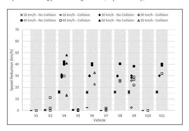
Testing for the obstructed running child (child pedestrian surrogate travelling at a speed of 5 km/h (3 mph)) scenario with a 50 percent overlap for the daylight condition found one
