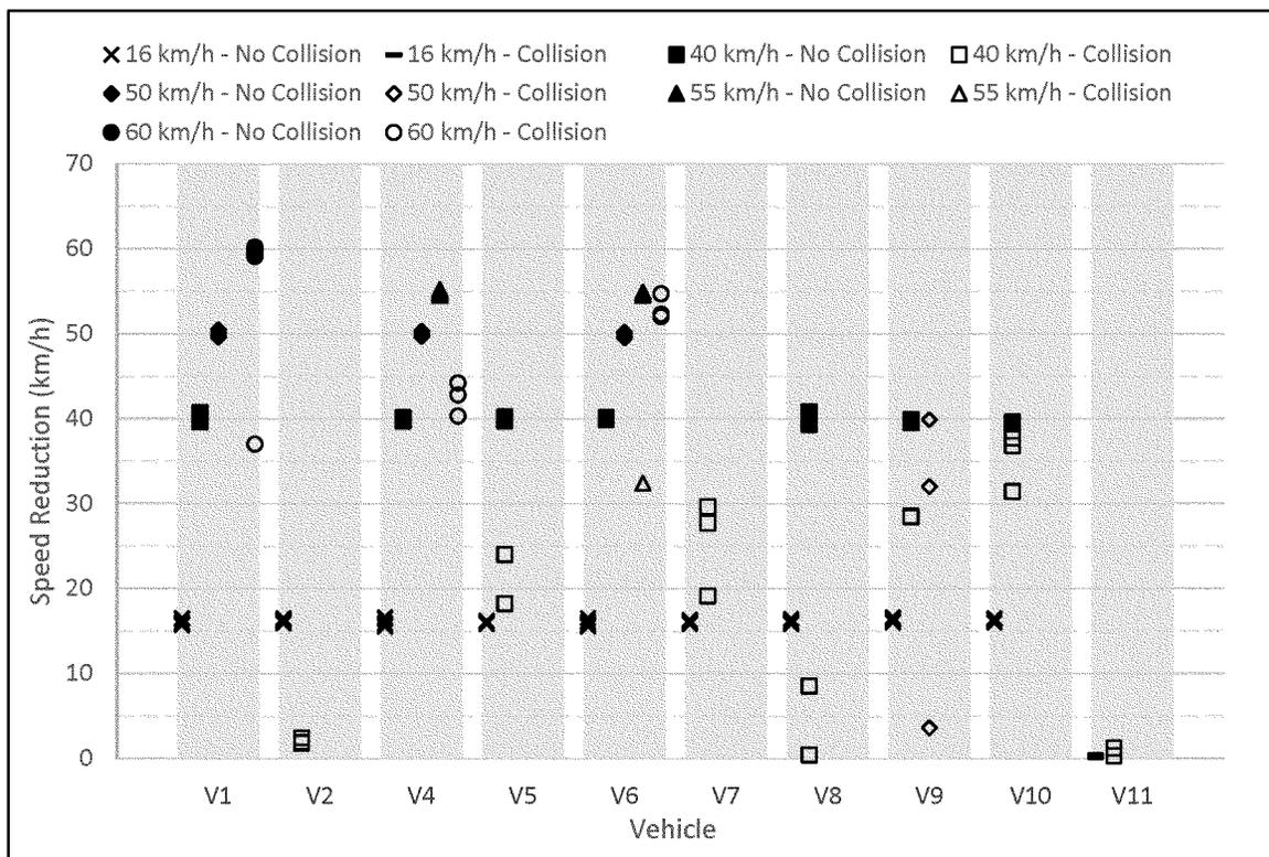
NHTSA upper beam testing using the stationary pedestrian along path scenario under dark lighting conditions resulted in one vehicle, V4, being able
