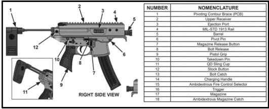
Parts of the "SIG MPX Copperhead" in the Sig Sauer Operator's Manual<sup>114</sup>
