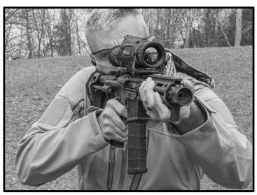
Example of firearm with thermal scope with eye relief that requires shouldering of the firearm in order to be used as designed.
