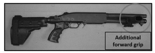
2014 submission of pistol grip firearm equipped with a "stabilizing brace" and forward grip
