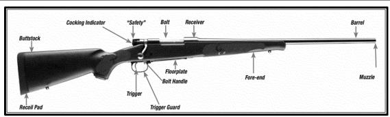
Parts of the "Winchester Model 70 Bolt-Action Rifle" in the Winchester Owner's Manual 109
