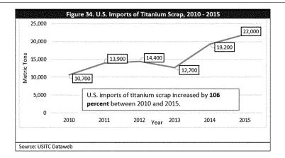
One reason for the increased use of scrap is the aviation industry's use of the "buy to fly" (BTF) ratio. The BTF ratio specifies the amount of titanium required to produce a given part. <sup>105</sup> For example, if the BTF ratio for a given part weighing one pound is 20:1, 20 pounds of titanium metal is required to produce the part weighing 1 pound. New developments in metallurgy and
