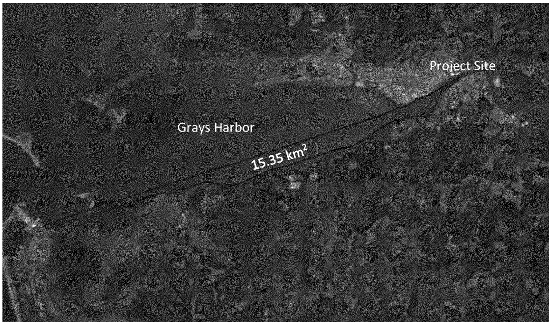
Figure 2. Estimated Area to be Ensonified to Level B Harassment Threshold for 48-inch Steel Piles
