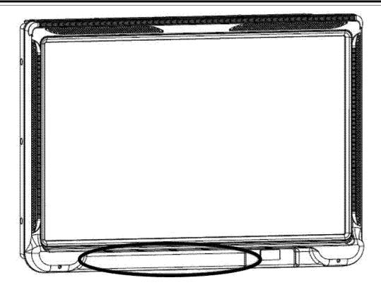
Figure 1 to paragraph (g)(1)(iii); placard location on bezel
