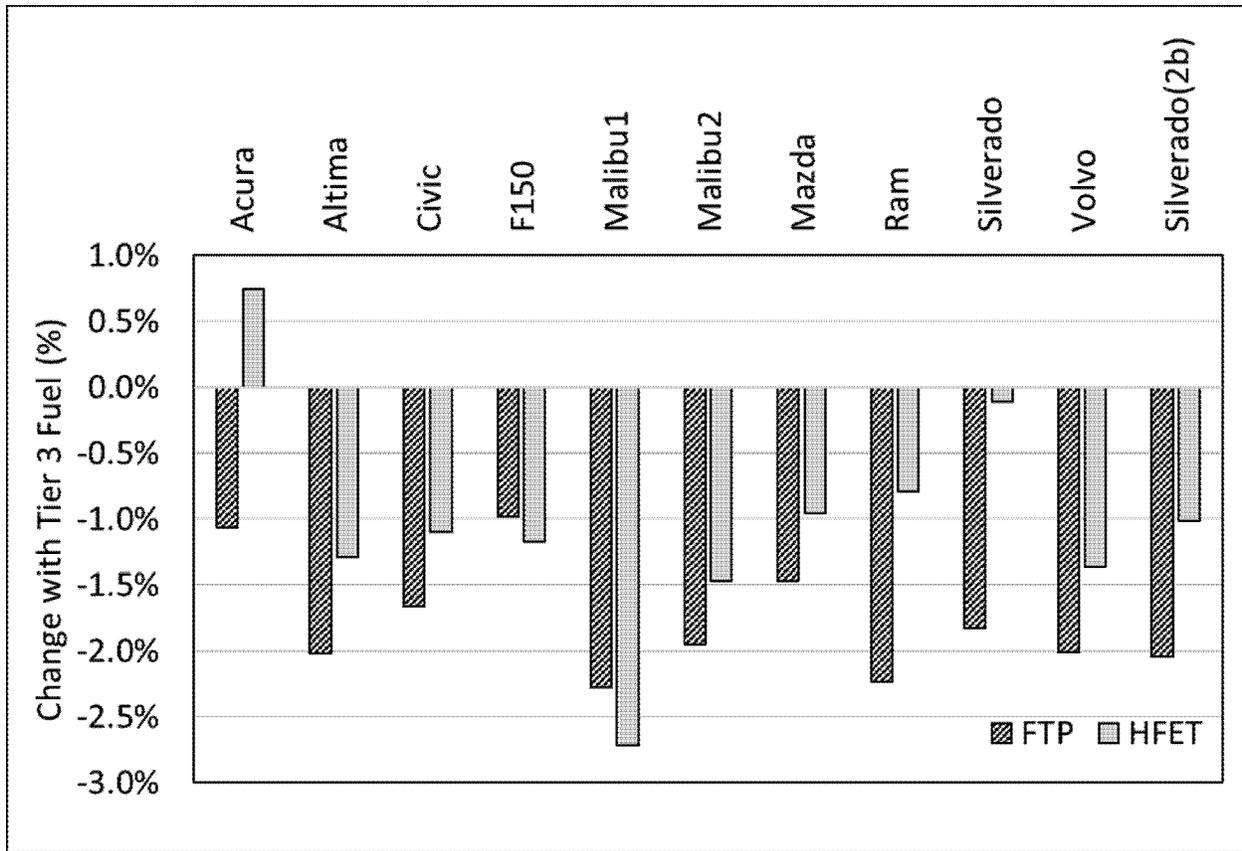
Figure III-1 Percent Change in CO<sub>2</sub> Emissions from Tier 2 to Tier 3 Test Fuel (%)
