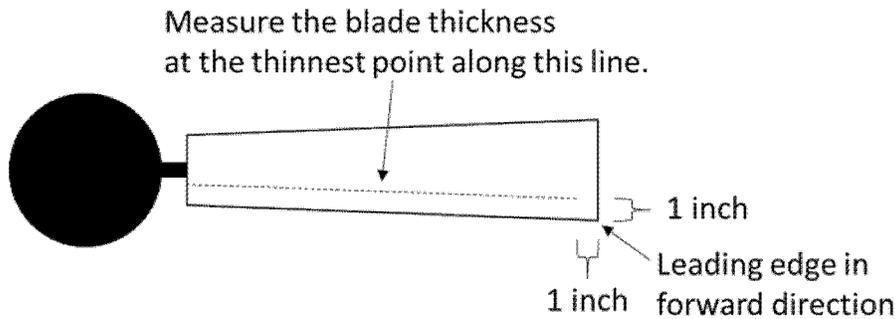
**Figure 1 to Appendix U to Subpart B of Part 430: Measurement Criteria for Fan Blade Edge Thickness**
