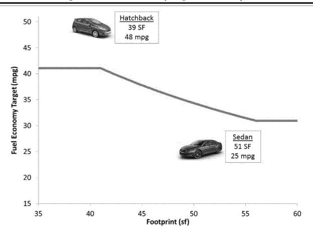
Figure X-1 - Illustration of Vehicle Models vs. Fuel Economy Targets
