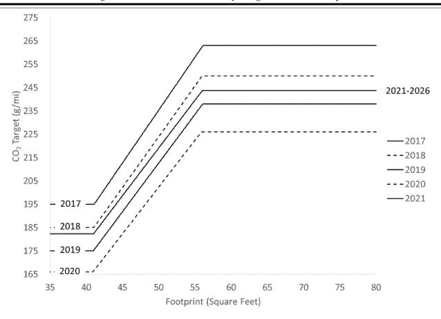
Figure III-2 - Passenger Car CO<sub>2</sub> Targets<sup>366</sup>
