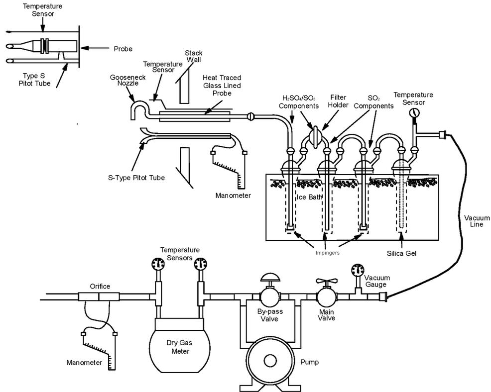
Figure 8-1. Sulfuric Acid Sampling Train
