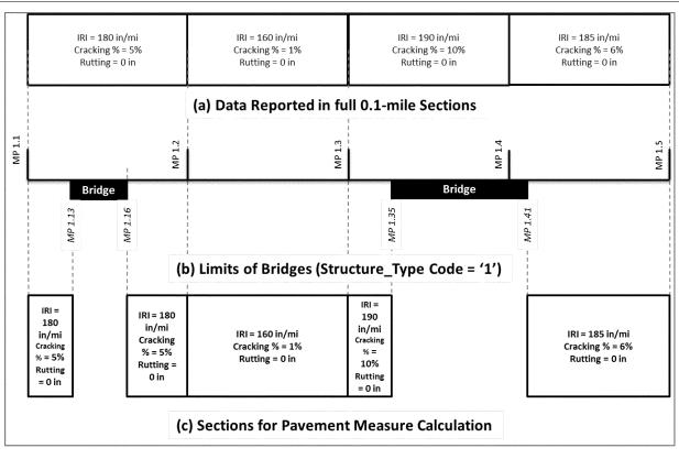
Figure 3 – An example of 0.10 mile pavement section with data measured in full 0.10 mile sections
