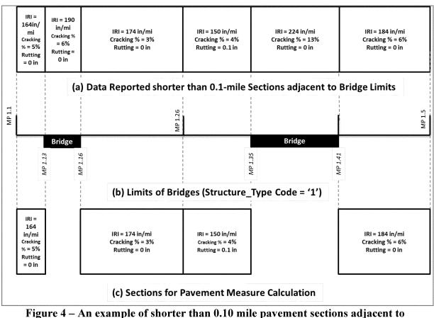
bridge limits where data is measured separately for each section
