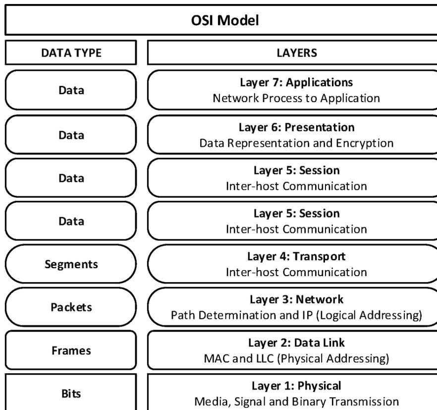
Figure III-5 OSI Stack
