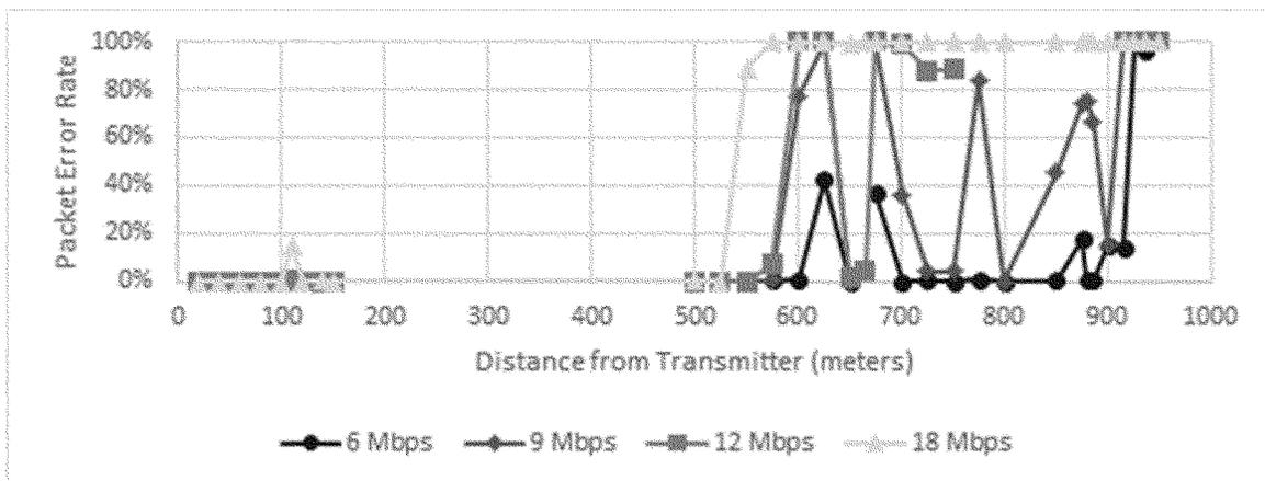
Figure III-3 Packet Error Rate based on Distance
