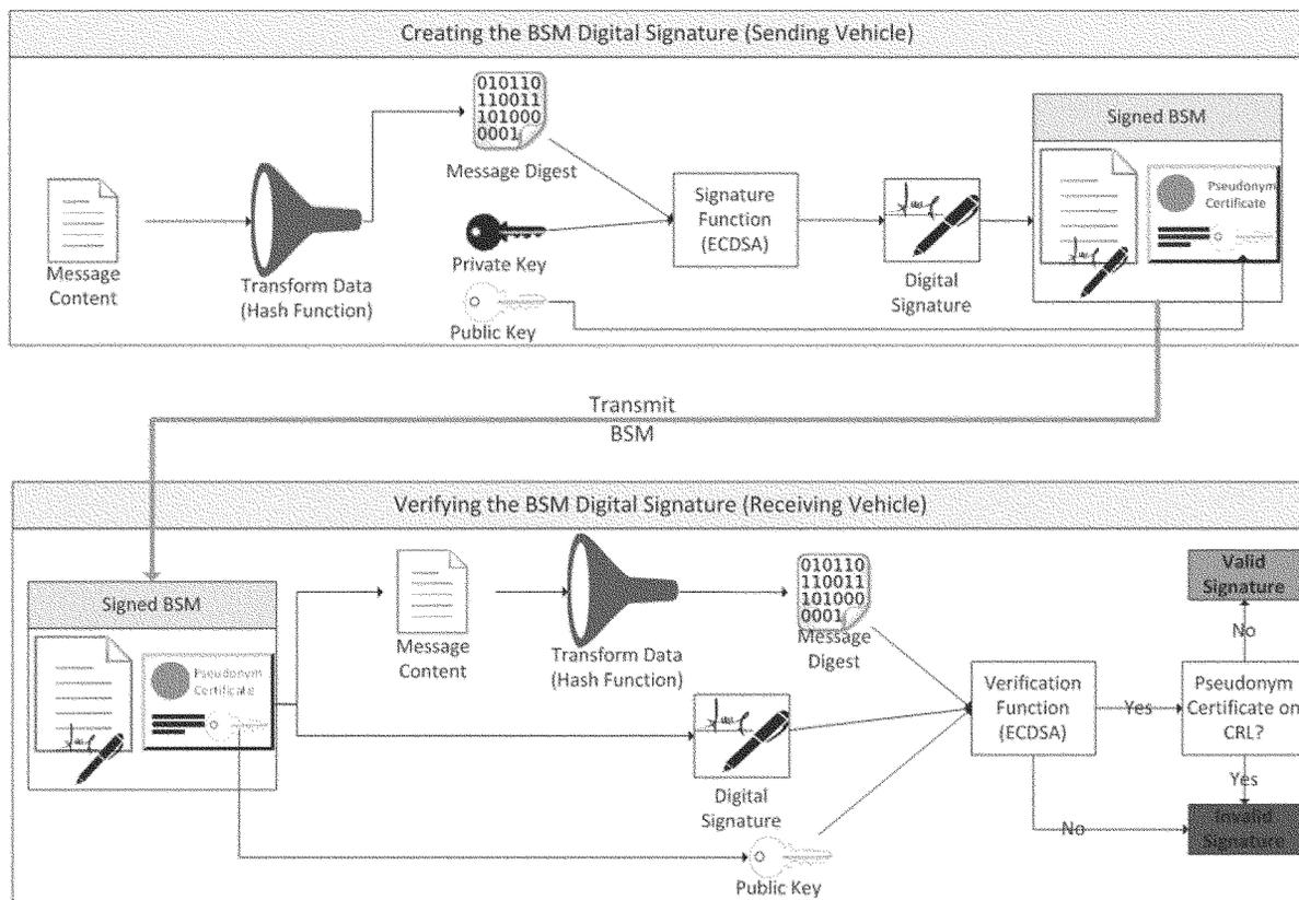
**Figure III-9 BSM Digital Signature Generation**
