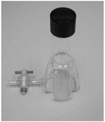
Figure 1. A Baffled Trypsinizing Flask
