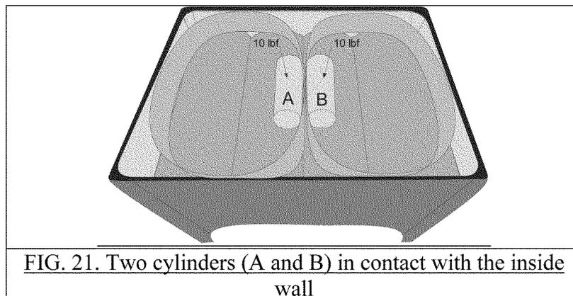
(GG) 7.10.2.11 Place 6" x 4" x 1/2" (152 x 101.6 x 12.7 mm) nominal thickness steel block weighing 3.3 lbs. (+/- 0.2 pounds) on the mattress panel on one side perpendicular to the longitudinal axis of the cylinder, with the centerline of the block adjacent to the midpoint of the cylinder. Place the block within 1/2" (12.7 mm) of the cylinder. If the block slides and touches either the inside wall or the cylinder, this is allowable.
