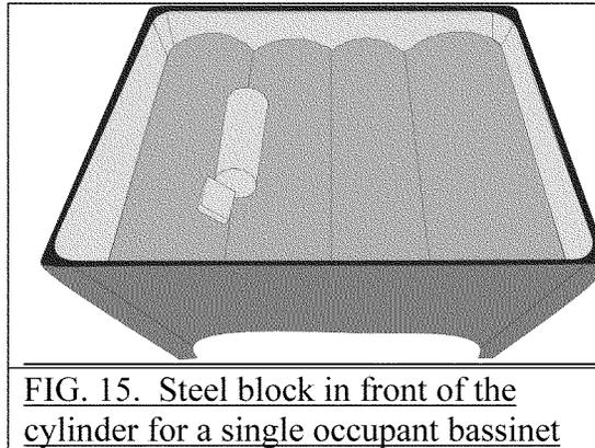
**FIG. 15. Steel block in front of the cylinder for a single occupant bassinet**
