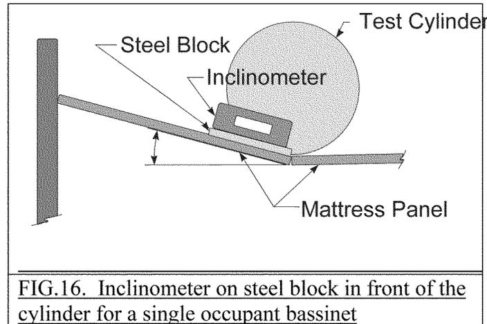
**FIG. 16. Inclinometer on steel block in front of the cylinder for a single occupant bassinet**
