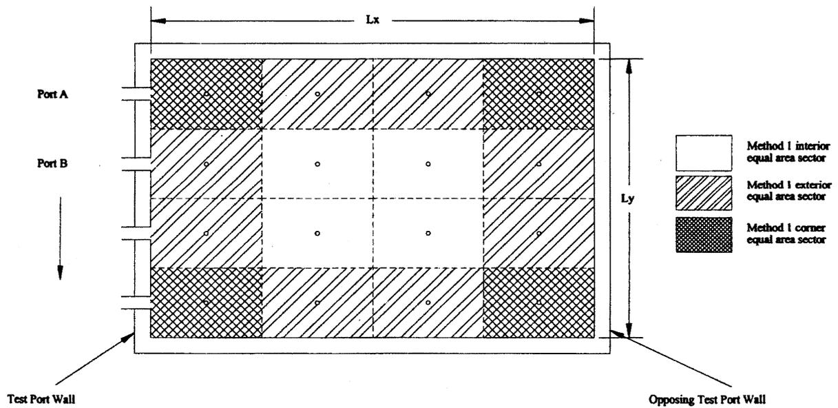
**Figure 2H-2. Method 1 Rectangular Duct Equal Area Sectors**
