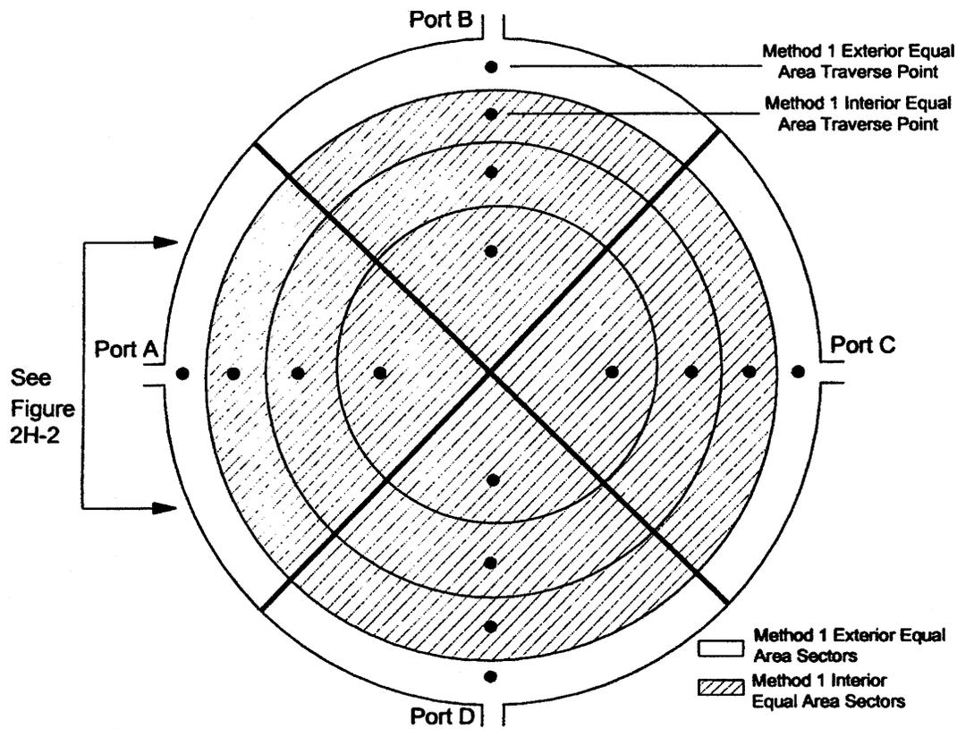
**Figure 2H-1. Method 1 Circular Stack Equal Area Sectors**
