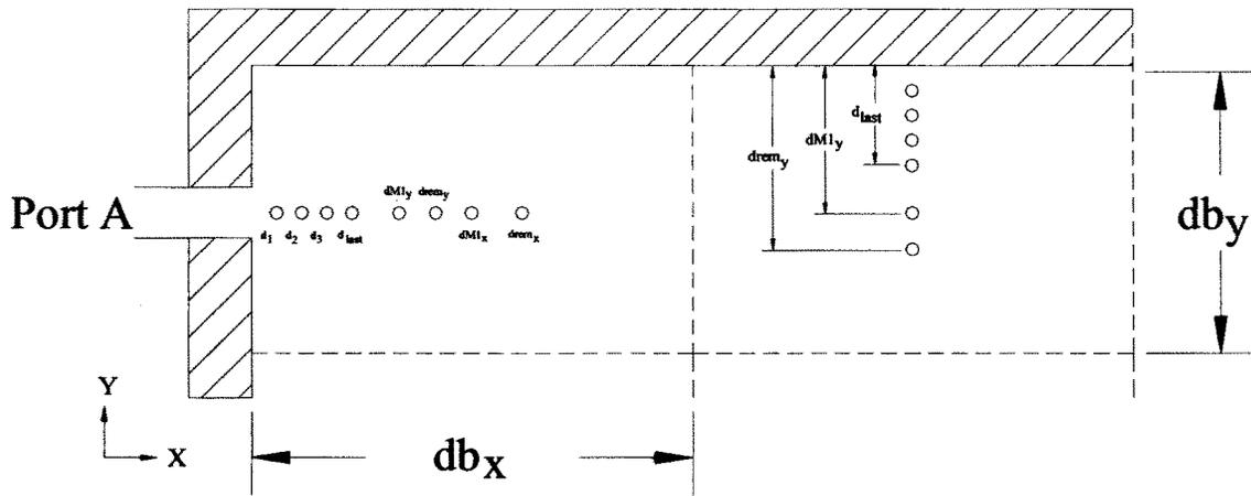
**Figure 2H-4. Rectangular Duct Wall Effects Traverse Points**
