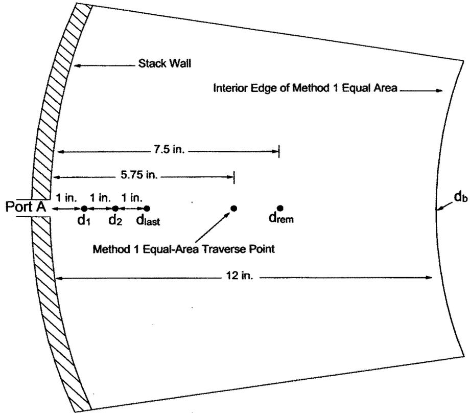
**Figure 2H-3. Circular Stack Wall Effects Traverse Points**
