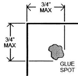
h. Continuous glue lines may be used as cover-to-cover seals on some designs (see 3.15.4 and 3.16.4), and must be placed along the entire length of the open edge and end no more than 3/4 inch from the open ends (see Exhibit 201.3.12.h)
