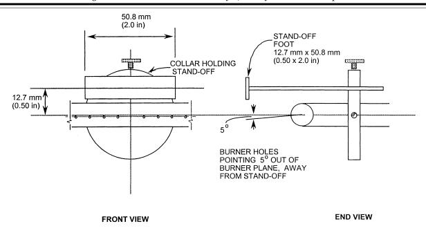
FIGURE 5. DETAILS OF BURNER STAND-OFF.
