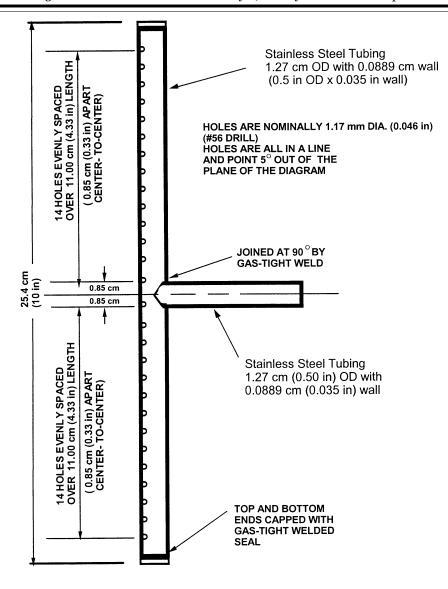
FIGURE 4. DETAILS OF VERTICAL BURNER HEAD.
