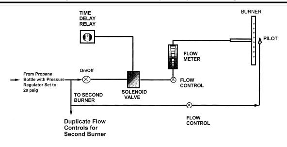
FIGURE 7. ELEMENTS OF PROPANE FLOW CONTROL FOR EACH BURNER
