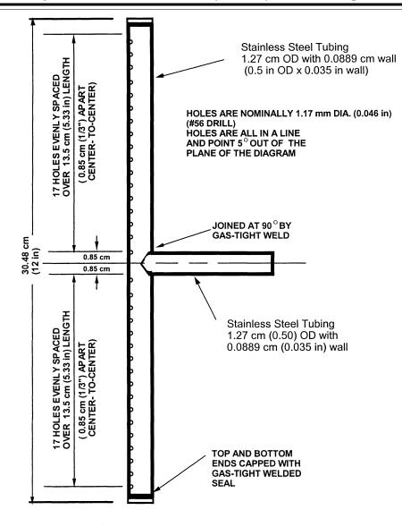
FIGURE 3. DETAILS OF HORIZONTAL BURNER HEAD.
