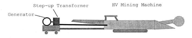
Figure 4-Power Source-75.829(c)(3) Generator Supplies 480/995 volts to step-up transformer for 2300 volts for tramming
