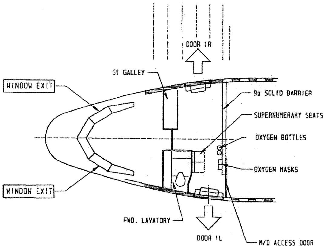
“Fig. 1: Emergency Exit Arrangement and 9g Barrier”
