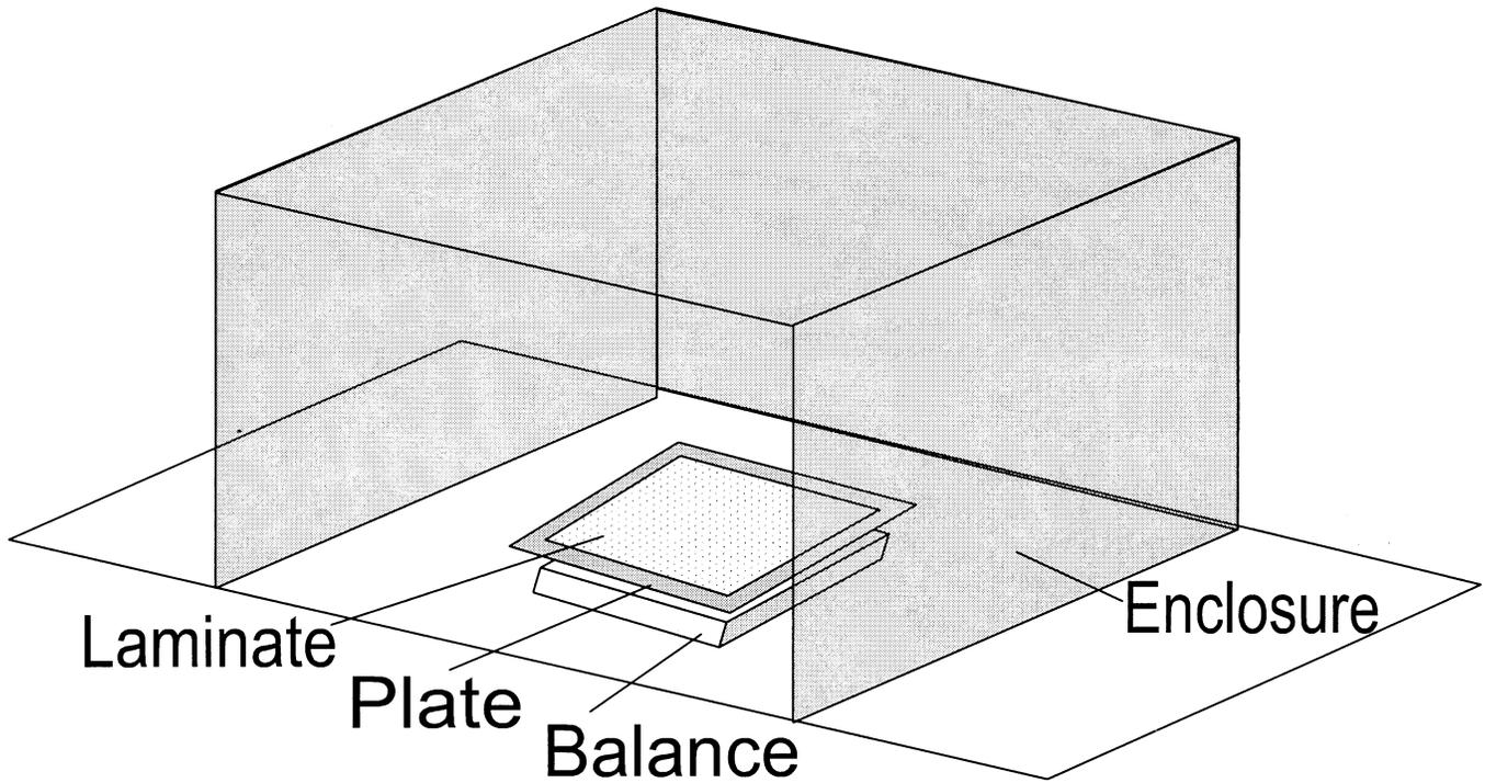
Figure 17.1. Typical Balance Enclosure
