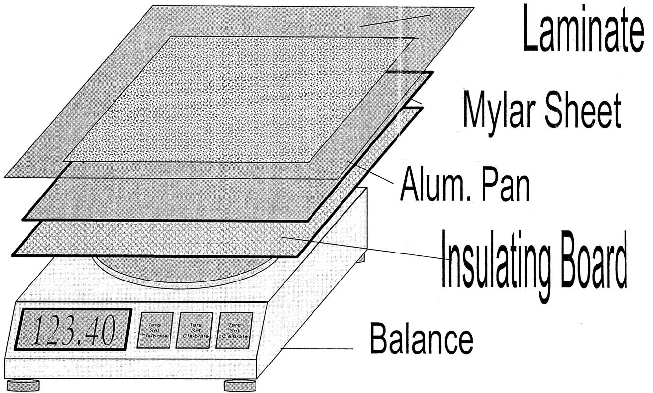
Figure 17.2. Scale, Plate, Insulating Board, Mylar, Laminate Order
