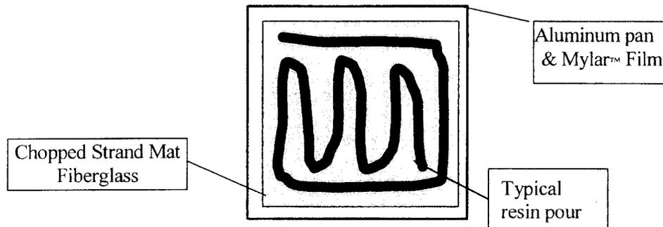
Figure 11.6 Resin Distribution Diagram
