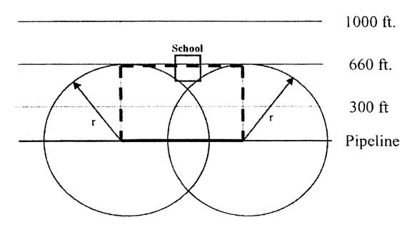
Note: This diagram represents the results for a 30" pipe with an MAOP of 1,000 psig.
