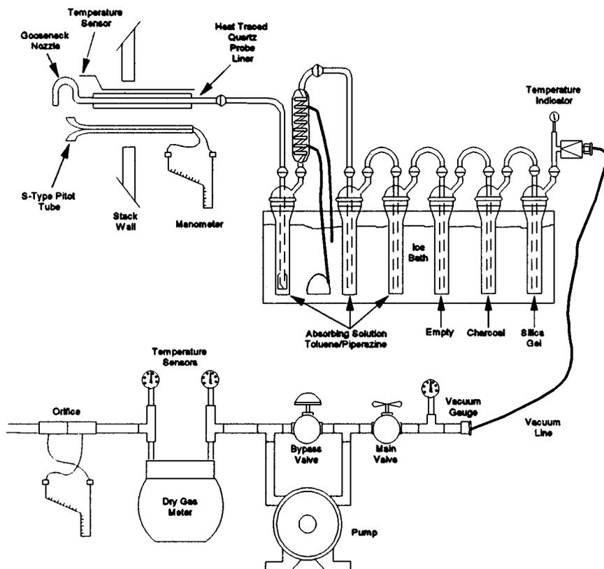
Figure 207-1-1. Sampling Train Configuration for Isocyanates
