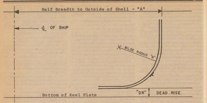
Note.—On an off-center lockage with the vessel touching the lock wall, the turn of the bilge will clear the lock-wall batters at the most critical point as shown in the Table of Limiting Drafts, subparagraph (d)(3) of this section.
