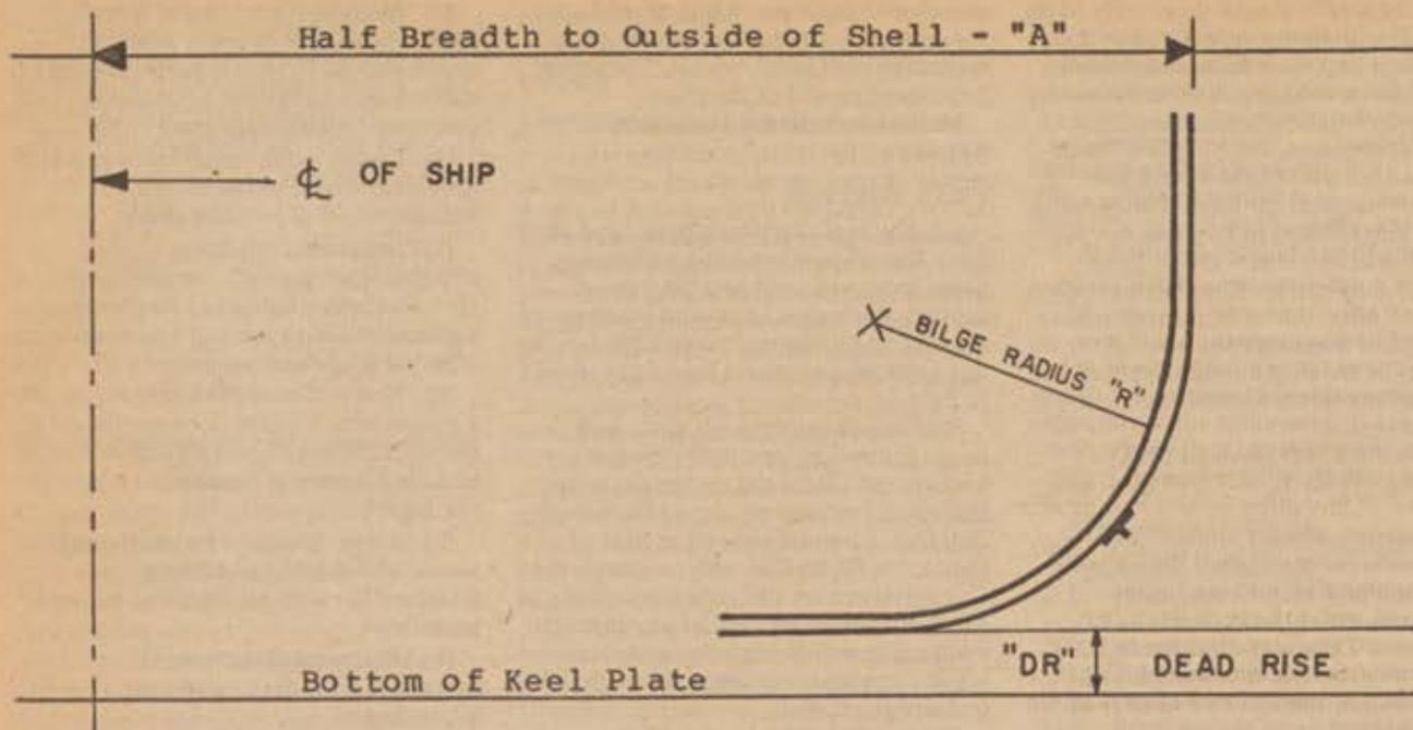
Note.—On an off-center lockage with the vessel touching the lock wall, the turn of the bilge will clear the lock-wall batters at the most critical point as shown in the Table of Limiting Drafts, subparagraph (d)(3) of this section.
