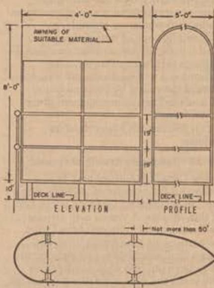
(c) Each platform is to be erected over the furthest forward point of the extreme beam at the waterline and not more than six inches from the vertical plane of shell plating. For vessels of unorthodox design requiring aft platforms, they shall be erected at a
