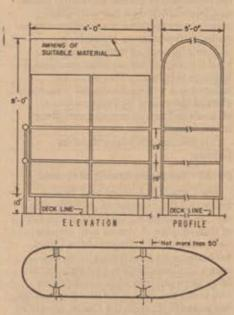
(c) Each platform is to be erected over the furthest forward point of the extreme beam at the waterline and not more than six inches from the vertical plane of shell plating. For vessels of unorthodox design requiring aft platforms, they shall be erected at a position which is approximately over the aftermost point of extreme beam at the waterline and not more than six inches inboard from the vertical plane of shell plating.
