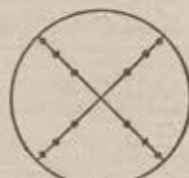
Figure 104-4. Cross section of circular stack showing location of traverse points on perpendicular diameters.
