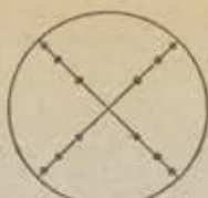
Figure 102-4. Cross section of circular stack showing location of traverse points on perpendicular diameters.
