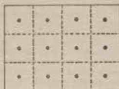
Figure 102-5. Cross section of rectangular stack divided into 12 equal areas, with traverse points at centroid of each area.
