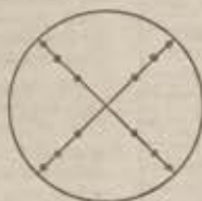
Figure 101-4. Cross section of circular stack showing location of traverse points on perpendicular diameters.
