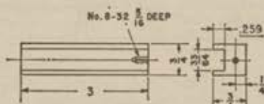
BURNER BODY GUIDE (1.9.) 2 REQ. ALUM.
