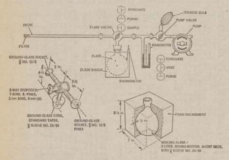
Figure 7-1. Sampling train, flask valve, and flask.
