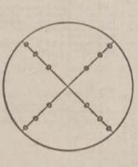
Figure 1-2. Cross section of circular stack divided into 12 equal areas, showing location of traverse points at centroid of each area.
