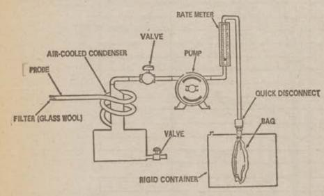
Figure 3-2. Integrated gas - sampling train.
