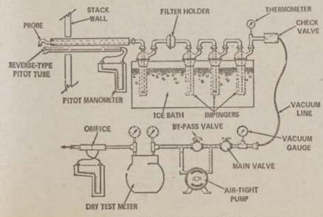
Figure 8-1. Sulfuric acid mist sampling train.
