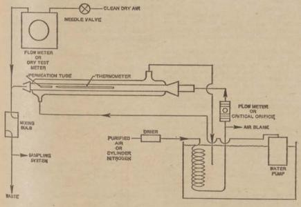
Figure 3. Permeation tube schematic for inboratory uses
