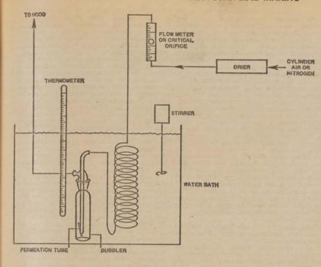
Figure 2. Apparatus for gravimetric calibration and field use.
