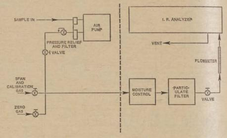
Figure 1. Carbon monoxide analyzer flow diagram.
