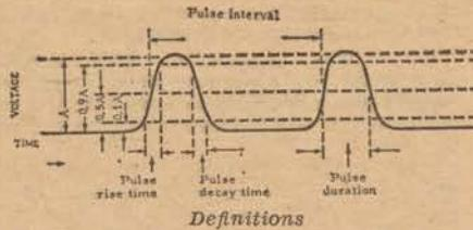
*Pulse amplitude A.* The peak voltage amplitude of the pulse envelope.
