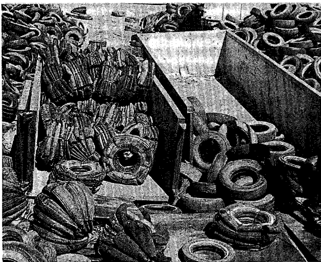
Twenty cubic yard industrial trash containers, or "dumpsters", are used to haul baled tires for short distances.
