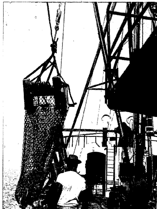
Figure 7. Clam dredges being hauled aboard R/V Silver Bay. (Bureau of Commercial Fisheries photo)
