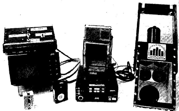
Figure 1. The VSPC system. The system includes the prism with an aluminum "skin", handles, radon lights, a CCD camera, waterproof housing and cable terminations, cable system, control panel, a 4" black and white SONY Watchman, a broadcast quality JVC mini-VHS VCR with audio dubbing, remote control, and 20 minute cassettes.
