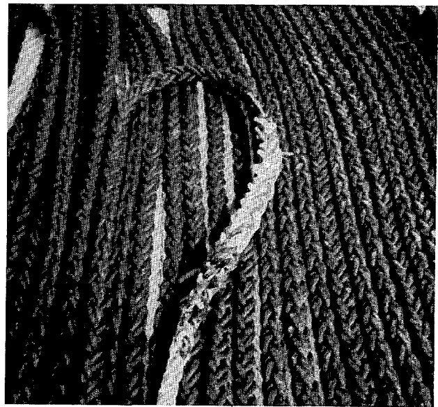
Figure 1. Nylon/Polypropylene Splice
