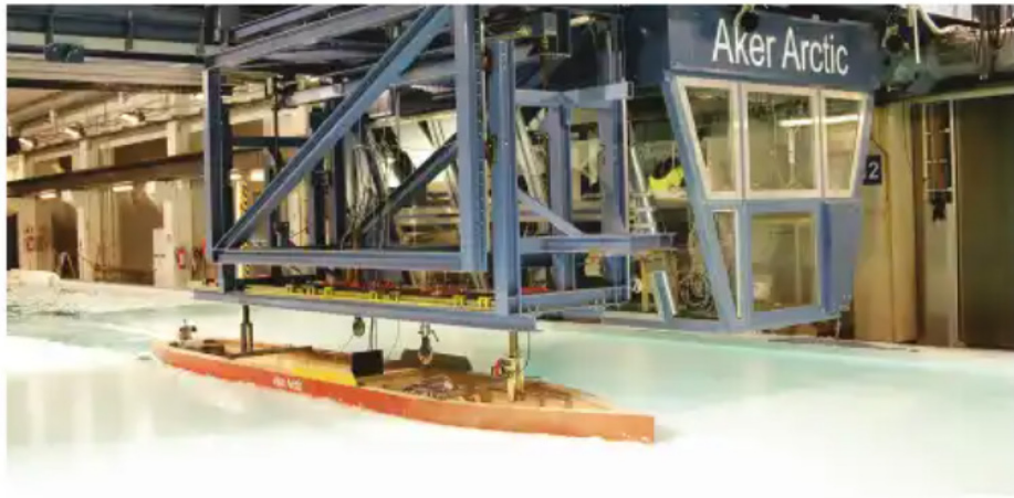
Figure 7: Ice Model Basin at Aker Arctic
