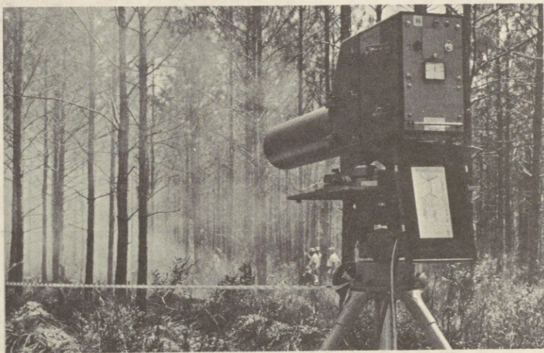
A backscatter transmission meter is used to monitor time changes in the density of a smoke plume from a prescribed burn in a Southern Pine forest. (U. S. Forest Service photo.)
