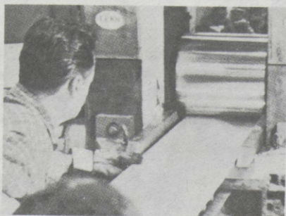
Silver strip being rolled at Englehard Industries plant for Kennedy 40% silver commemorative coin.
