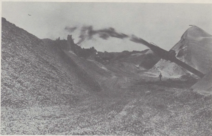
Chips are propelled into position for storage. There is constant movement as an inventory of wood residues await utilization as pulp, kraft paper and container board for export and for domestic manufacture into bags, containers and wrapping paper.
