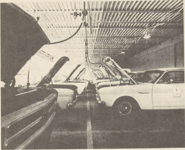
Fig. 6 - Operational fleet during "time loading" refueling process
