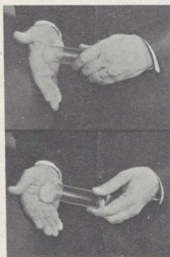
The secret of Palm-N-Turn: apply 12 pounds of pressure against the palmed cap and turn counterclockwise approximately 54 degrees. This sequence has proved frustrating to small children.
