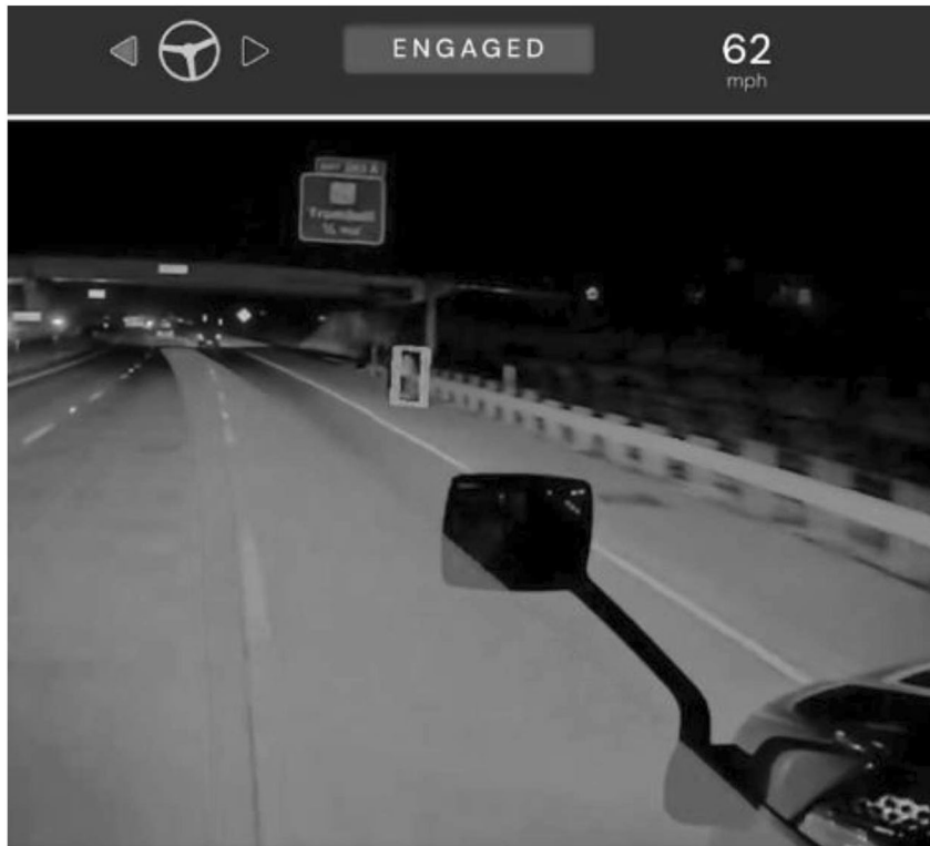
A Kodiak autonomous truck recognizes a pedestrian on a highway from over 130m away at night, shifting to another lane to give the pedestrian extra space. 26
