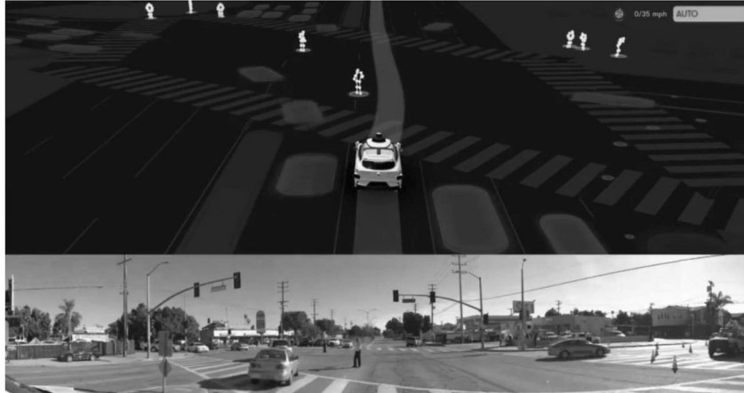
A Waymo vehicle recognizes and adheres to a police officer directing traffic at a Los Angeles intersection. 25
