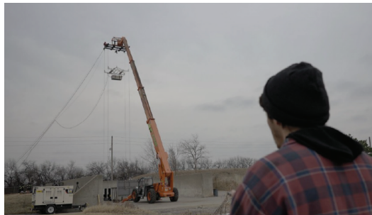
BETA partners with NIAR and FAA to conduct first-ever 50-foot drop test of full-scale battery system.
