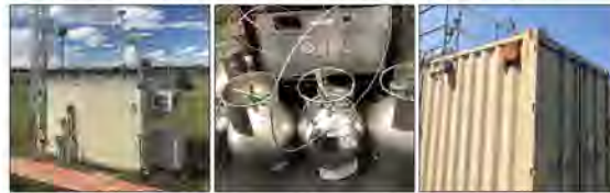
(Left to right) National Core network (NCORE) monitoring site; canisters used to collect samples for measuring air toxics; near-road monitoring site.
