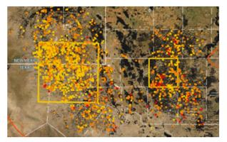
Figure 2. Survey of methane emissions in 55,000 km<sup>2</sup> of the Permian Basin, Fall 2019. White: < 2 kg/h; Yellow: 2-100 kg/h; Orange: 100-1000 kg/h; Red: > 1000 kg/h. Environmental Defense Fund PermianMAP/UArizona/NASA Survey 1 [EDF, 2021b; Cusworth et al., 2021].
